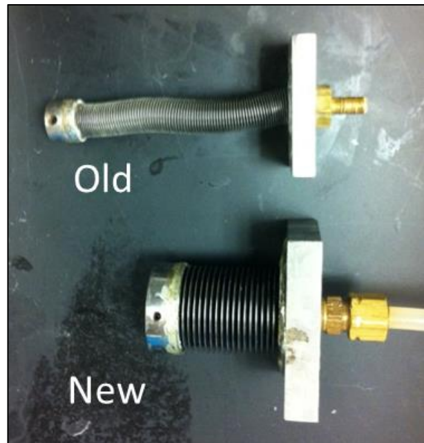
Figure 13: Size comparison of old and new driving bellows.
